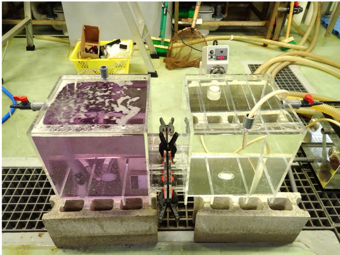
Fig. 2. Two end tanks joined. Water was injected into the upstream tank (right) with a peristaltic pump. The water flow velocity in the joint pipe was adjusted to approximately 1 mm per second. Note that the dyed water in the downstream tank (left) does not penetrate into the upstream tank (right).
