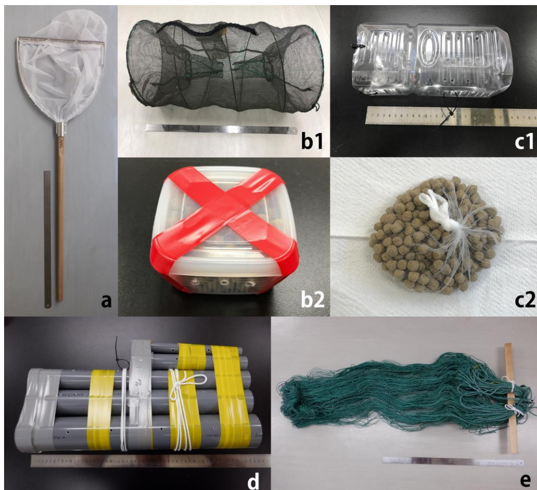
Fig. 1. D-framed net and traps used for capture. a: D-framed net; b1: cage trap (conger eel cage trap); b2: bait for b1; c1: plastic bottle trap; c2: bait for c1; d: PVC pipes; e: seaweed net (trap using a cultured seaweed net).
